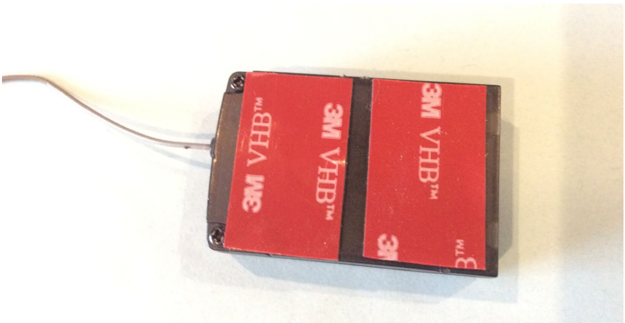
Turnigy Receiver: Place double sided sticky tape on the bottom of the receiver.
